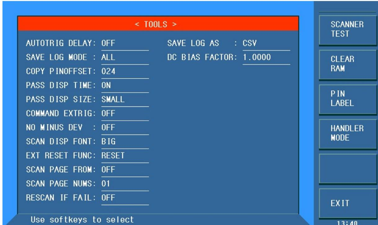
If necessary, select the softkey PIN LABEL to access the <TRANSFORMER PIN LABEL> page. Here you can enter the names of the transformer pins at the corresponding pin positions if they are not numbered „normally“.
